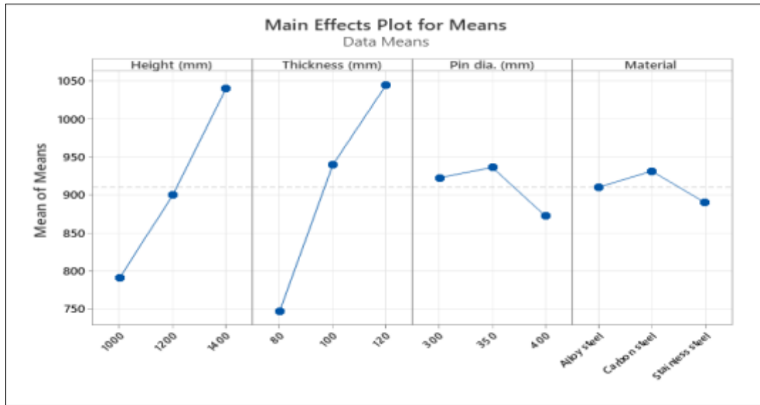
Figure 2 Main effects plot for the mean performance displacement, FOS, and stress. Across different levels of design factors. The plot shows the influence of Height, Thickness, Pin diameter, and Material on the output response
