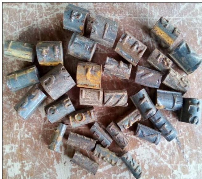
Figure 2 20 mm cut sizes of steel bars for hardness analysis
