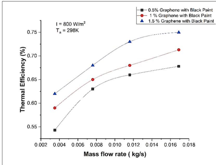
**Figure 3** Thermal Efficiency vs mass flow rate for different absorber plate coating
