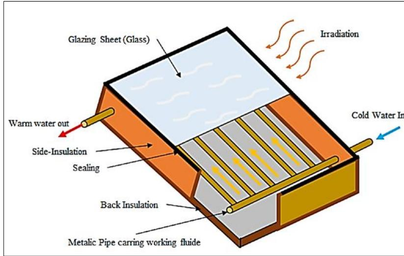
**Figure 1** Diagram of flat plat solar heater
