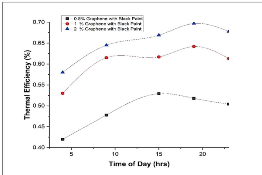
**Figure 4** Comparison between Thermal Efficiency (%) of Solar air heater with different percentages of graphene embedded in black paint vs time of day (hrs)
