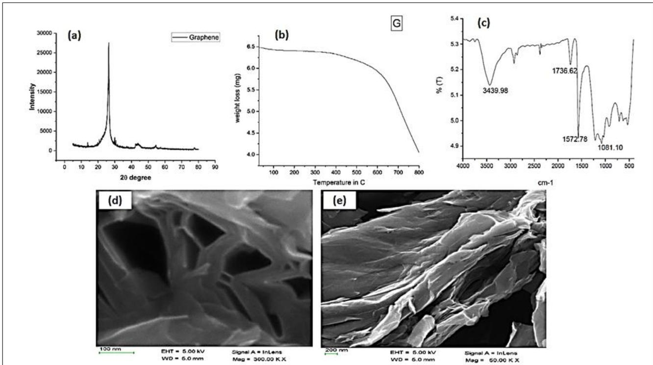
**Figure 2** (a) The X-ray diffraction analyses of the graphene powder, (B) Thermogravimetric analysis (TGA), (c) Insulation resistance test (IR), and (d-e) Scanning electron microscopy of graphene powder
