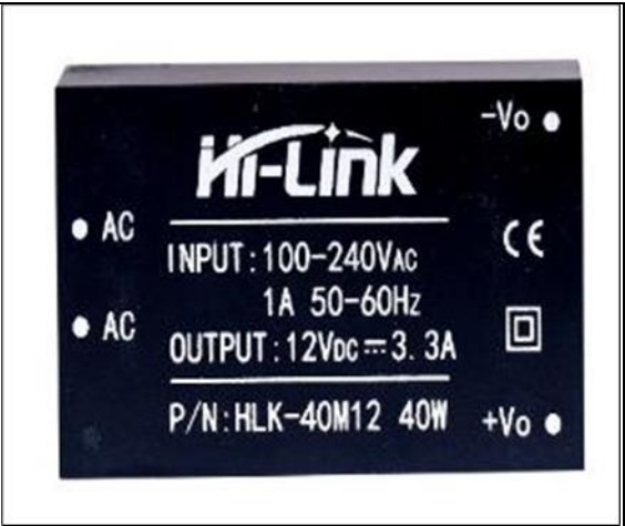
Figure 4 Hi-Link power supply convert 230V AC to 5V DC for ESP32
