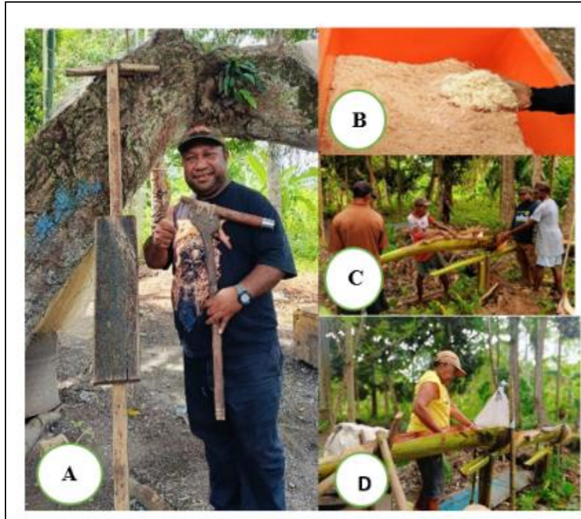
Figure 3 A. Grater and scraper tools for sago pith; B. Pith ready for extraction; C. Construction of starch water filtration channels and sedimentation area; D. A woman extracting (pressing) sago pith, allowing the starch to settle in a collection container
