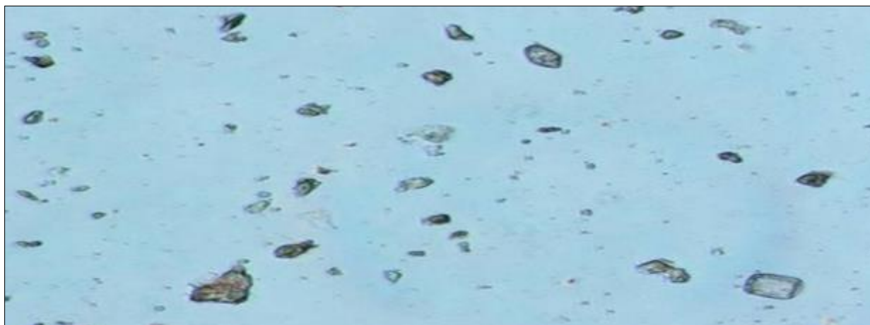
Figure 2 Green synthesized MgO nanoparticles observed at 40X through Phase Contrast Microscope
