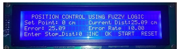
Figure 5 LCD 40 x 4 Character Display
