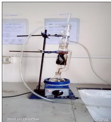
Figure 4 Soxhlet Extractor with the thimble inside.
