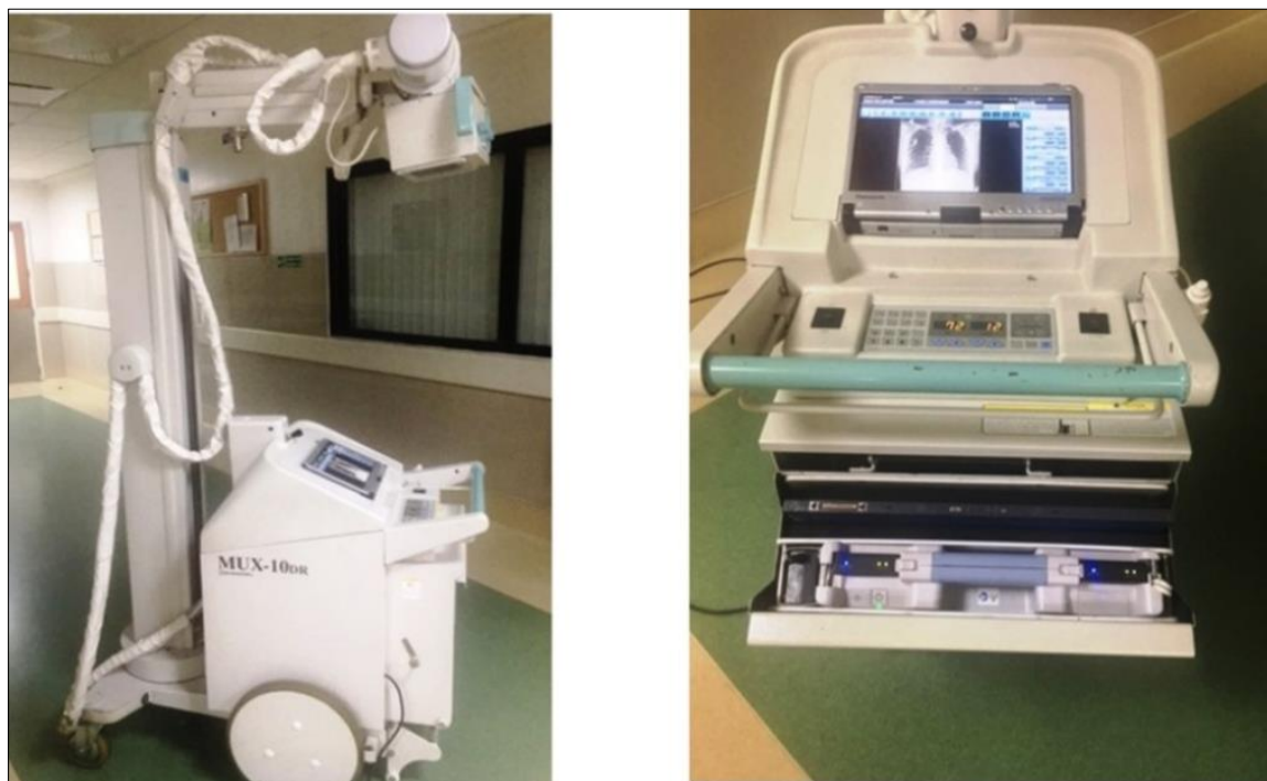
Figure 2 The retrofitted wireless network-based digital portable radiography system. (Courtesy-on-site portable DR, Ruby Hall clinic, India)
