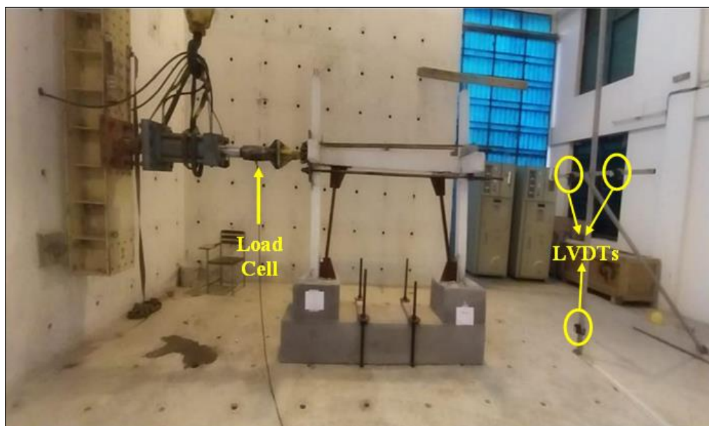
Figure 6 Test Setup and Instrumentation
