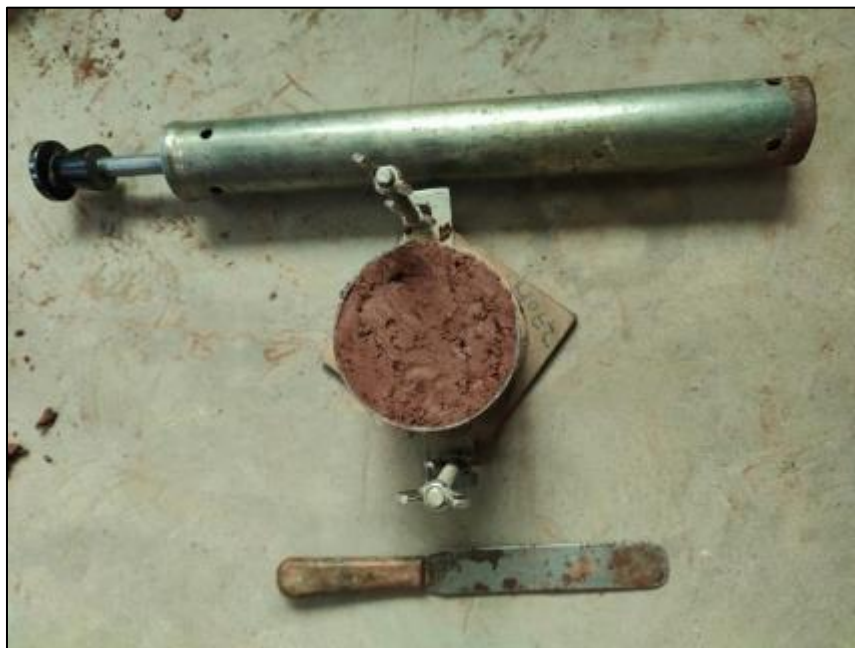
Figure 9 Standard Proctor Test of Natural Soil
