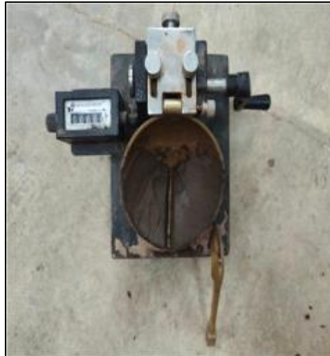
Figure 6 Liquid Limit test in Progress
