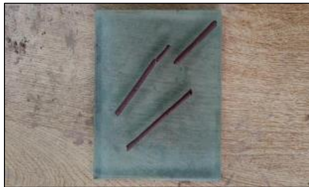
Figure 7 Plastic Limit Test in progress
