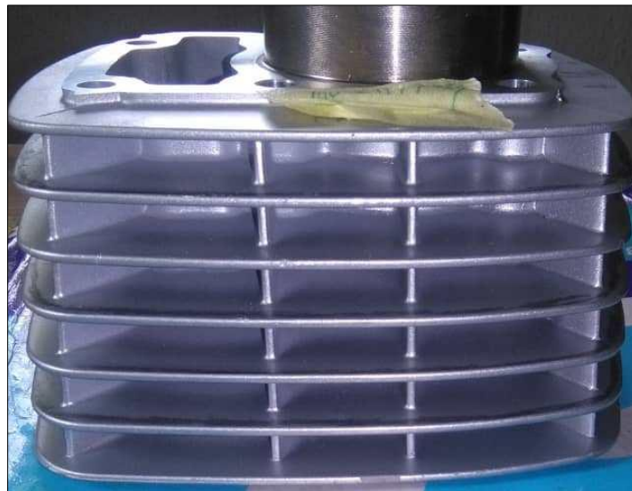
Figure 1 Control Model: ERRAND 125 CT (Original motorcycle Engine block or Heat sink (Rectangular Engine Block, Original Sample)
