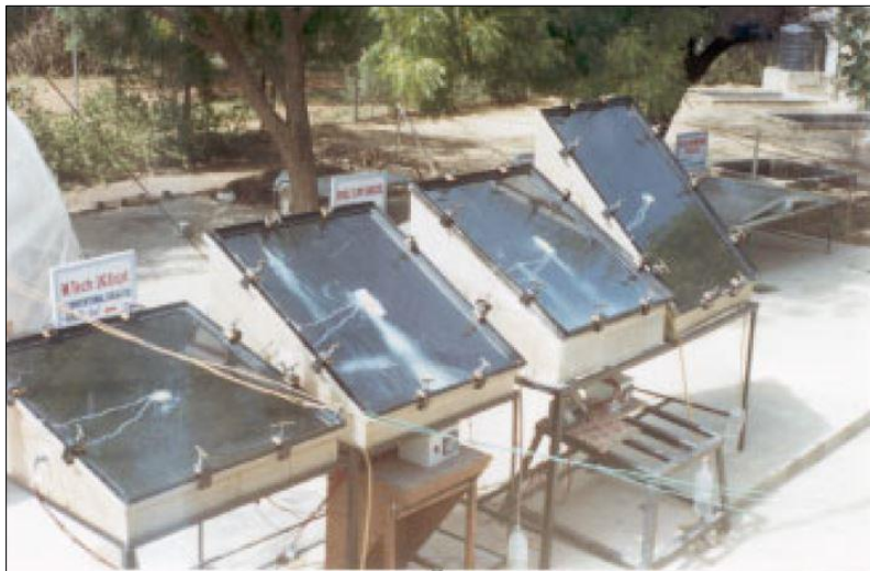
Figure 1 Working stills with covers inclinations 15, 30, and 45° from left 1st, 2nd, and 4th [6]
