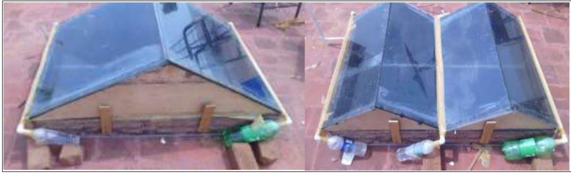
Figure 3 DSSS and multi slope still studied by [12]
