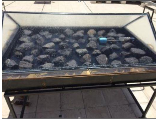
Figure 5 DSSS with basin covered with rocks used by [15]
