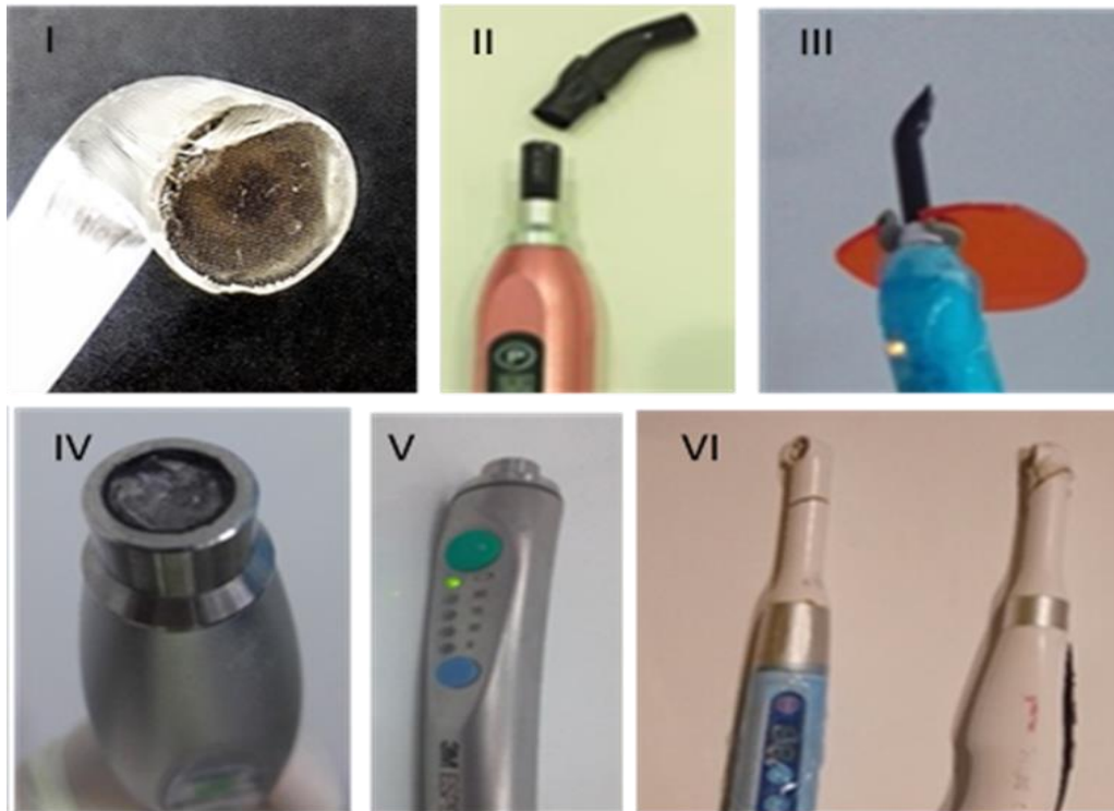
Figure 2 The Light Guide Conditions: I) Chipped light guide tip. II) & III) Fractured light guide tip at varying levels. IV) Fractured external part of the light guide. V) Missing light guide. VI) Fractured plastic cover
