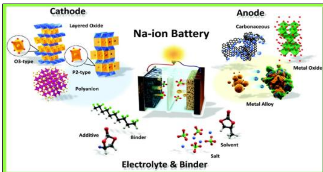
Figure 2 A typical sodium-ion battery showing various impacting materials components (15)
