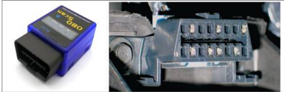
Figure 5 O.B.D-2 scanner and a standard 16-pin diagnostic connector [24-25]
