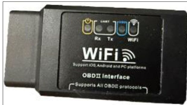
Figure 6 ELM327 scanner with Wi-Fi and Bluetooth compatibility
