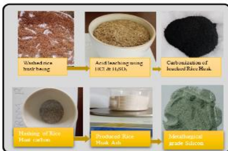
Figure 3 A schematic process for the preparation of silicon from raw rice husk
