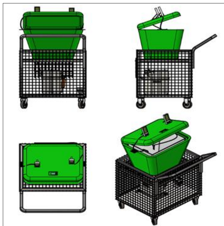
Figure 4 Orthographic projection of the cold storage system
