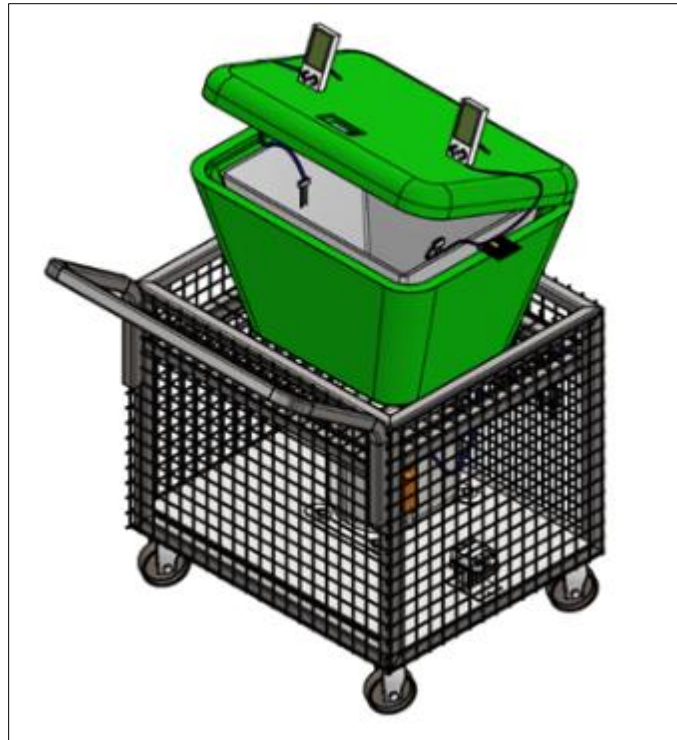
Figure 3 Isometric projection of the cold storage system
