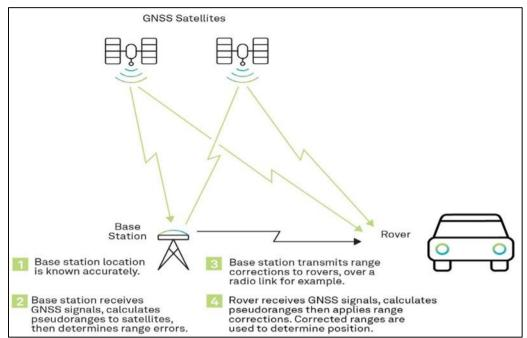
Image copied from Figure 41 Differential GNSS (DGNSS) Overview (Extracted from Chapter 5 Resolving Errors-Differential GNSS(DGNSS)) of the 3rd edition of the book: Industry Experts from Hexagon | NovAtel (28 March 2023), "An Introduction to GNSS. A primer in using Global Navigation Satellite Systems for positioning and autonomy." Published by Hexagon | NovAtel, https://novatel.com/, https://novatel.com/an-introduction-to-gnss/resolving-errors/differential-gnss, accessed on 1 December 2024.
