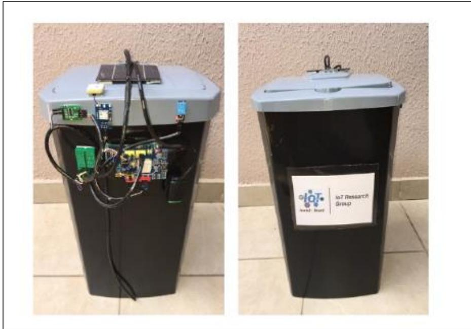
**Figure 3** Waste Bin Prototype
