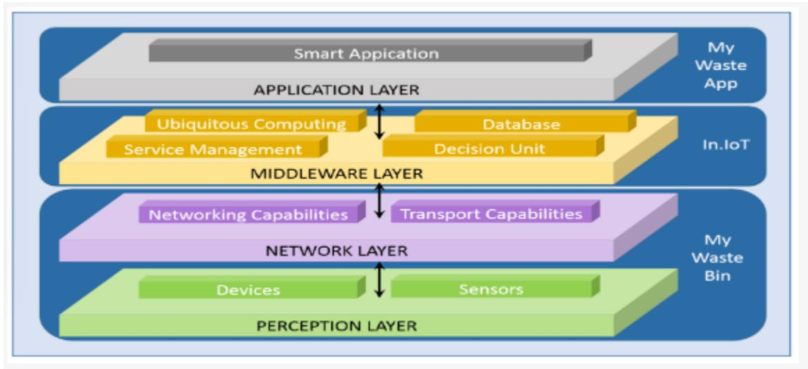
**Figure 1** Architecture for the waste management System
